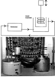
Fig. 7. Paste stirring vessel
